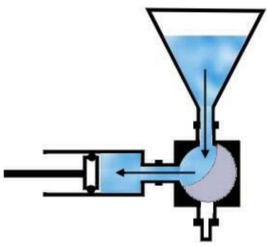
II. The valve Rotor (pallet) shifts position, and the piston moves the product from the cylinder to the filling nozzle and into the container.
