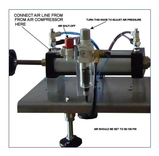
The Fillmaster has been designed to operate on demand. In other words, a fill cycle is initiated when the operator presses the foot pedal. The machine will go through and complete one fill cycle and then automatically shut off until the foot pedal is pressed again. The machine will operate as fast as the operator can get an empty container under the nozzle and press the foot pedal (filling the container).
