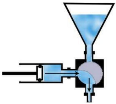
III. The valve Rotor (pallet) shifts to to its original position, cutting off the flow of product.
