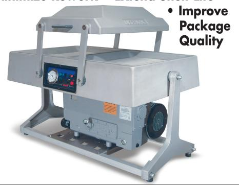
If you're faced with any of the above challenges, Koch Equipment's Ultravac 2100 swing lid double chamber vacuum packaging machine is your solution. With more than 3,000 machines in use the Ultravac 2100 is the best selling American made vacuum chamber machine.
