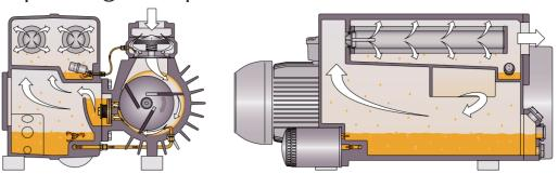
The vacuum pump works on the rotary vane principle.
