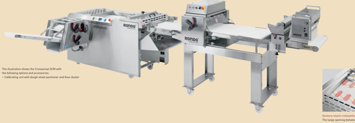
The large opening between the guillotine and rotary table enables you to place ham, salami or slices of cheese on the triangles of dough.
